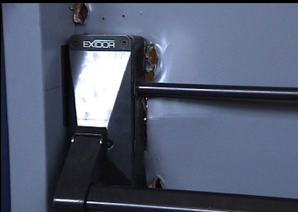
Inside view after 10 mins and the 4th bolt is still holding the door secure.
