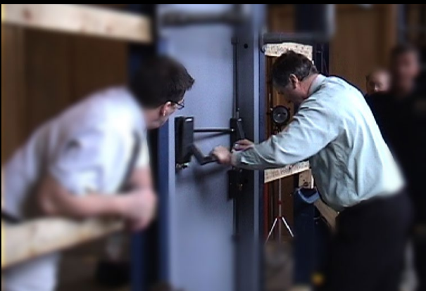
Inside view after 20 mins and the mechanism has jammed preventing entry.
